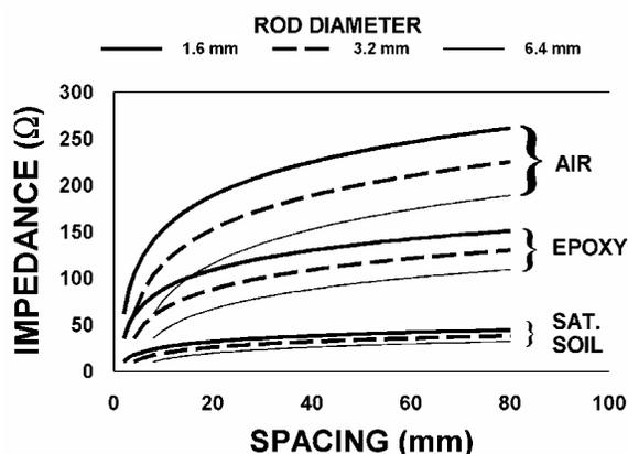
**Figure 4.** Influence of rod spacing, rod diameter, and permittivity of the medium on impedance of the waveguide according to Eq. 6. Permittivities are: AIR, unity; EPOXY, close to 3; and SATURATED SOIL, approx. 35.
