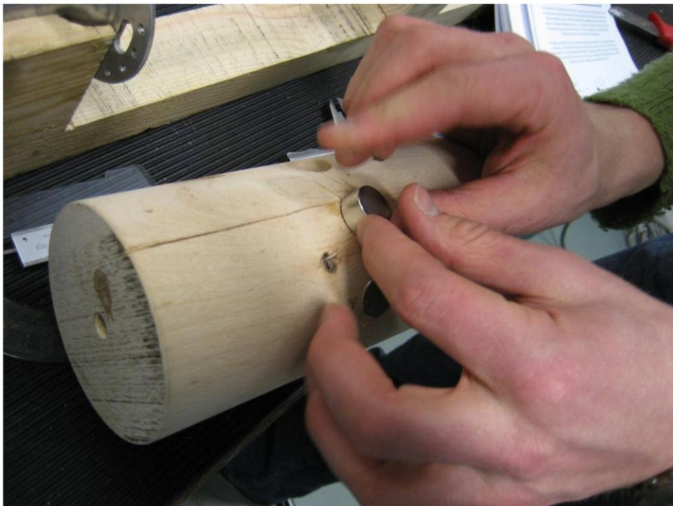
**Picture 4: Inserting the magnets**
