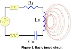
Where  $L_R$  = Inductance of the antenna.  $C_R$  = Value of Tuning capacitor.  $R_s$  = Series resistance of the antenna.
