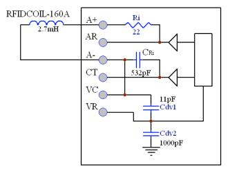
Antenna drive with RFIDCOIL-160A @ 134.4khz
