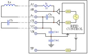
Figure 6. Antenna Drive Interface
