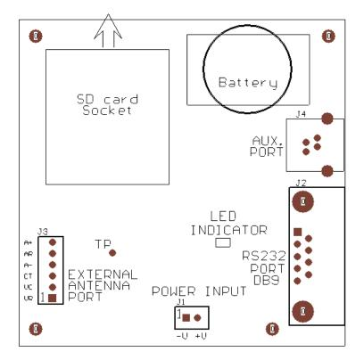
Fig 2. Main Unit connector diagram.
